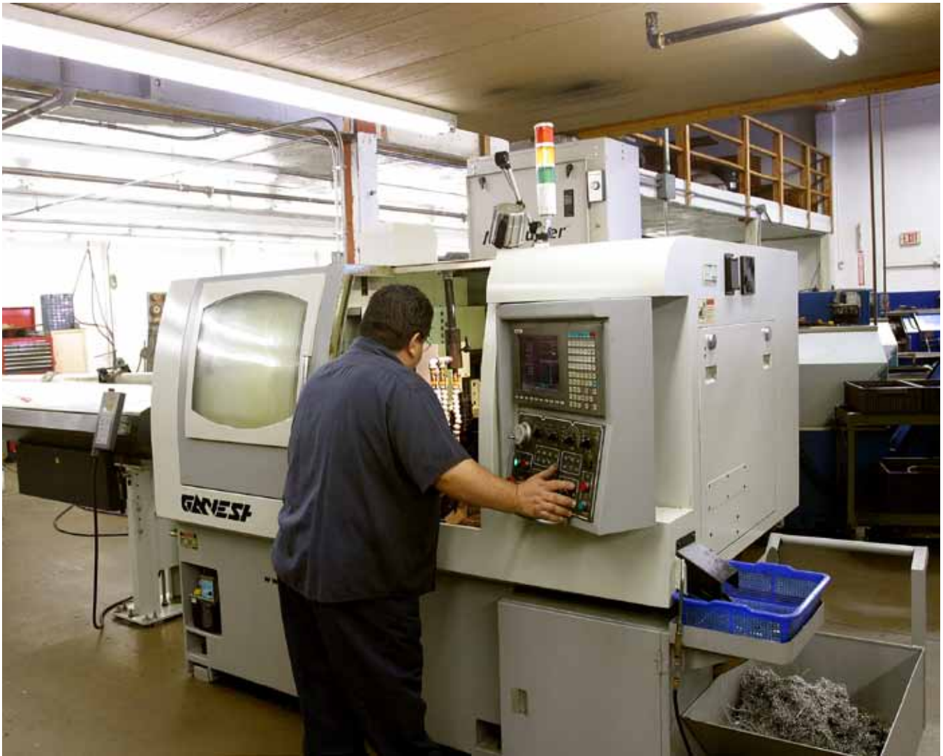
CNC lathe operator Carlos Sandoval sets up the Ganesh Cyclone-32 CS 7-axis twin-spindle CNC turn-mill center with 11 live tools and 27 total tools. The Ganesh is the workhorse for Heather, bringing in business from other shops without multi-axis capability.
