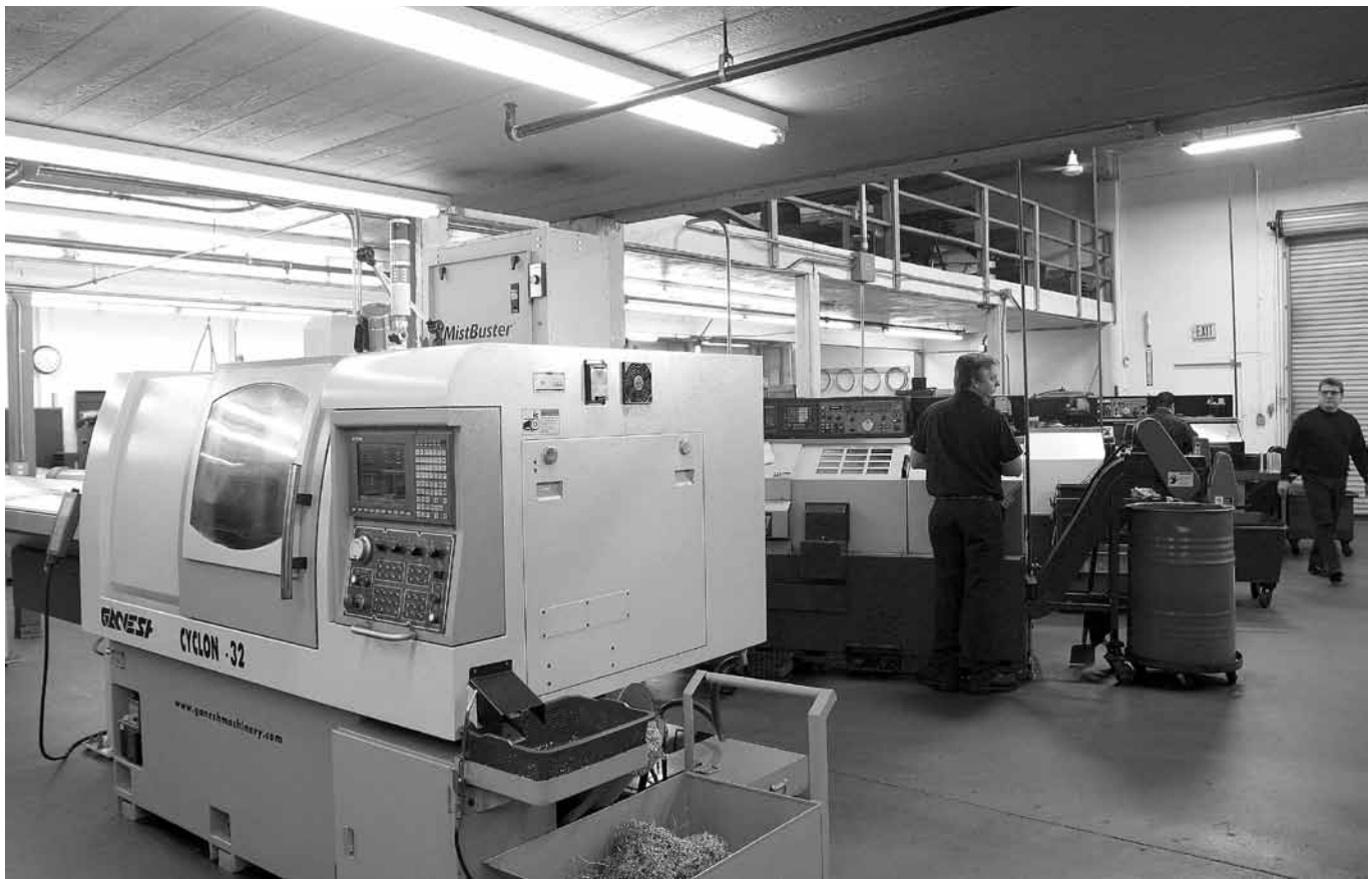
Line up of machines at Heather Screw Products. In the foreground is the Ganesh Cyclone 32, with live tooling and bar feeder. In the background are three Femco Durga 25E lathes. CNC lathe operator is Rafael Vargas.
